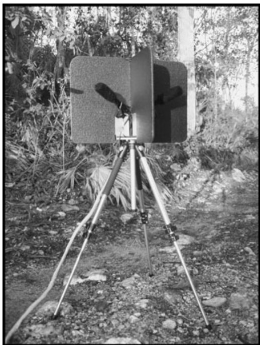
Fig. 1. Photograph of SRS four-microphone recording system.
